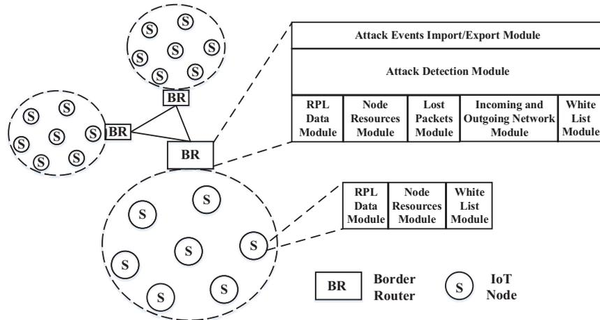
Figure 1. Proposed IDS Block Diagram.
