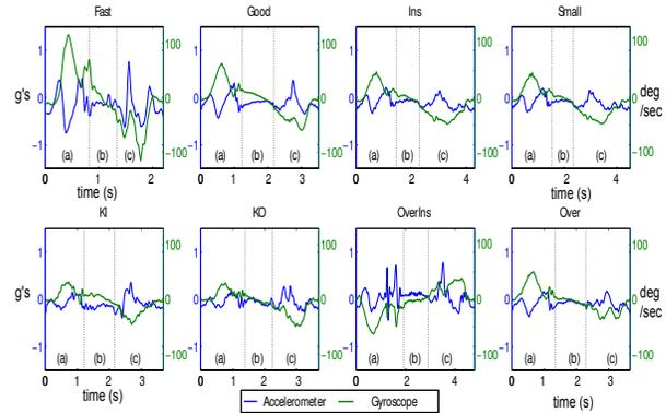
Figure 2. Accelerometer and gyroscope raw data from WIMUs for different labels.
