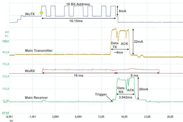
(c) Oscilloscope trace for radio events
