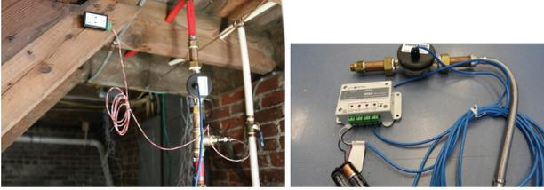
Figure 3: An inline water sensor (bottom) with attached data logger collects second granularity data on water drawn from the hot water tank (top) in the test home.
