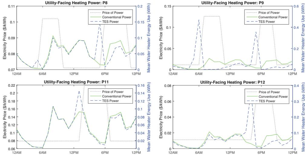
Figure 10: Heating TES just before peak hours to minimize standby loss can create a "new peak" in water heating just before peak hours. However, the magnitude and time of this peak depends greatly on the pricing scheme. In widespread use, such prices could be adjusted to suppress this peak or move it to times of excess power generation (e.g. renewables).
