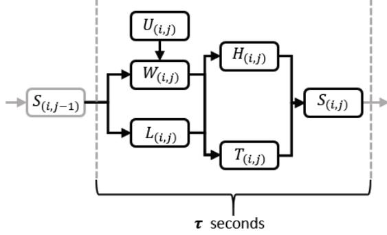
Figure 2: ThermalThrift predicts the state of the tank  $S_{i,j}$  through a series of modeling constraints. The predicted hot water use  $W_{i,j}$  is calculated from historical use  $U_{i,j}$  and the previous tank temperature  $S_{i,j-1}$ . Thermal losses  $L_{i,j}$  are also calculated from  $S_{i,j-1}$ . These losses  $T_{i,j}$  are then used to predict the heating requirement  $H_{i,j}$  and the final tank temperature  $S_{i,j}$  for the  $\tau$  second interval.
