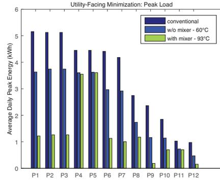
Figure 9: With a human tolerable TES limit of 60°C requiring no mixing valve, ThermalThrift shifts 24% of the peak load. For some pricing schemes no more shifting is possible (e.g. P4-5), but on average a 93°C TES limit shifts far more of the peak load (62%).
