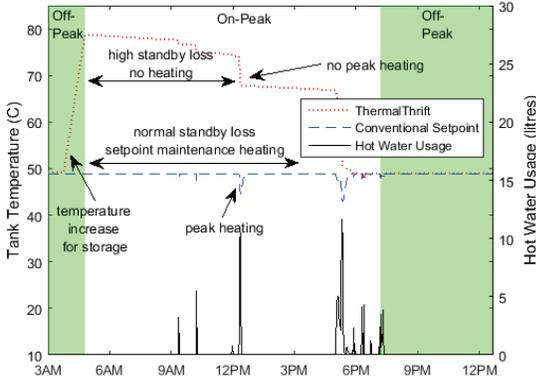
Figure 1: ThermalThrift stores thermal energy in off-peak hours (solid, edges) in preparation for usage during peak hours (white, center). ThermalThrift prevents the purchase of energy during peak hours while higher temperature stored energy is available. A conventional water heater purchases energy during the entire peak period.
