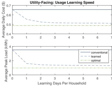
Figure 8: ThermalThrift is able to quickly learn usage patterns and successfully use predictions to manage standby loss. After only 7 days of training data for a given household, ThermalThrift is able to achieve within 5% and 36% of the optimal cost and peak load reduction.
