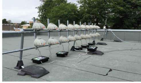
Figure 3: ELM sensors on top of WACL building
