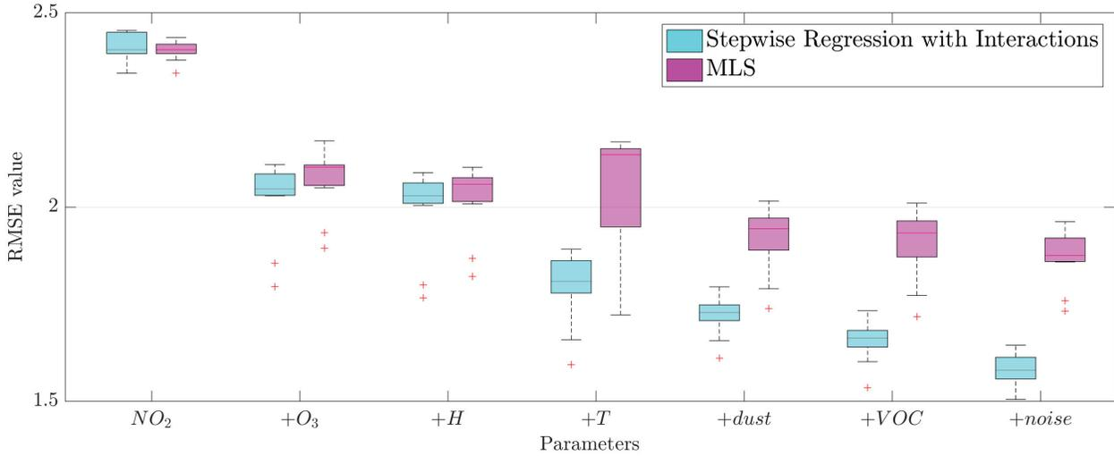
Figure 4: Calibration of a sensor in WACL
