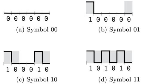
Figure 1: **Representation of the chip sequences and corresponding signals for the case of two bits per symbol and six chips per data bit.** Symbols 00 and 11 are the ones used in *μcode* to represent zero- and one-bits respectively.
