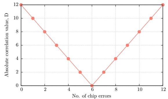
Figure 6: **Absolute correlation values as a function of the number of chip errors for  $N = 12$ .** The values decrease as the number of chip errors increases.
