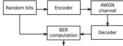
Figure 2: **Block diagram of the simulation framework.** In each run of the simulation, we encode a large number of random bits, transform the resulting chip sequences with an AWGN channel, and then decode them again.
