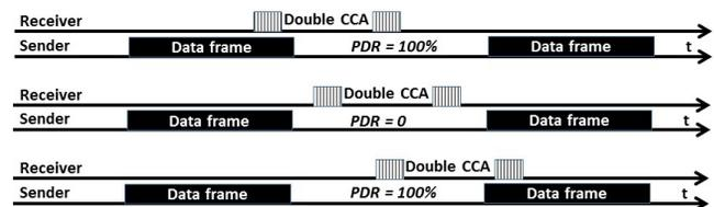
Figure 1. Effect of slightly different clocks on the PDR (the receiver clock is faster in this example).
