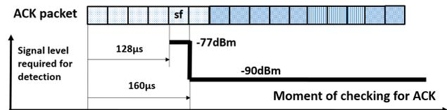
Figure 2. ACK detection levels.
