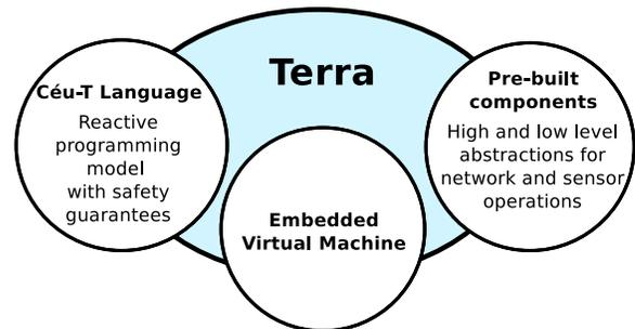
Figure 1. Terra system basic elements.
