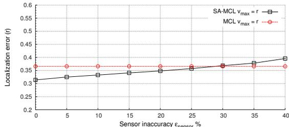
Figure 9: Localization error for different sensor precisions.
