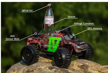
Figure 12: Fully assembled RC car mobile node.
