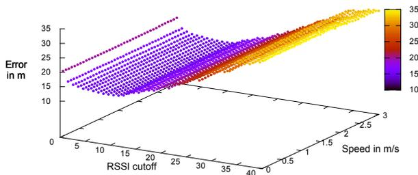
Figure 20: Absolute MCL error with varying parameters.
