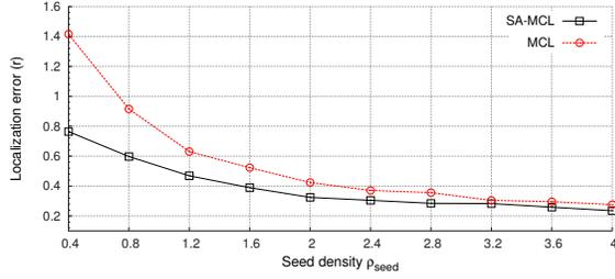
Figure 5: Localization error for different seed densities.
