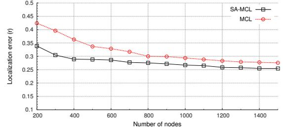
Figure 7: Localization error for different amounts of nodes.
