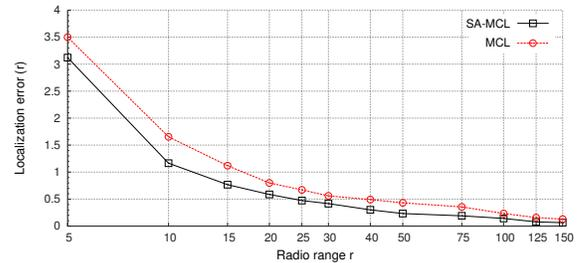
Figure 8: Localization error for different radio ranges.
