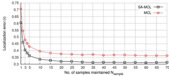
Figure 6: Localization error for different sample set sizes.
