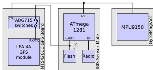
Figure 10: Data bus connections on the mobile node. Power supply lines not shown.
