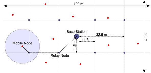
Figure 15: General field test setup.
