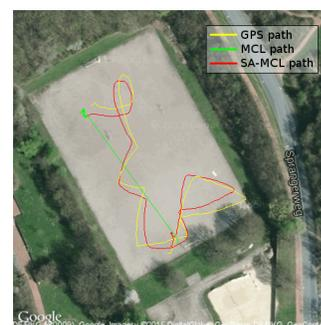
Figure 18: Path taken by RC car during experiment.
