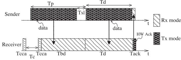
Figure 3. Unicast transmission in ContikiMAC.
