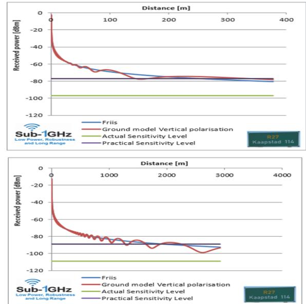
**Figure 1. Link budget and Range expectations for (a) 2.4GHz and (b) 868MHz deployments**
