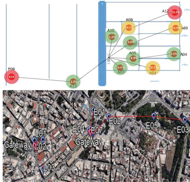
**Figure 2. Network topology for (a) indoor and (b) outdoor deployments**
