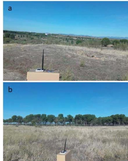
Figure 6. Vegetation effect: PDR=85 % for node in a and 68 % for node in b.
