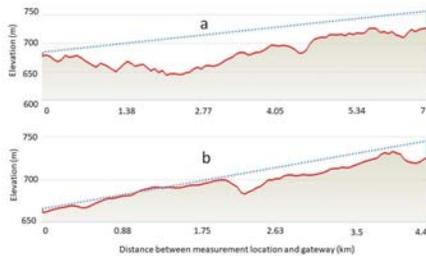
Figure 5. LoS comparison: PDR=100 % for node in a and 0 % for node in b.
