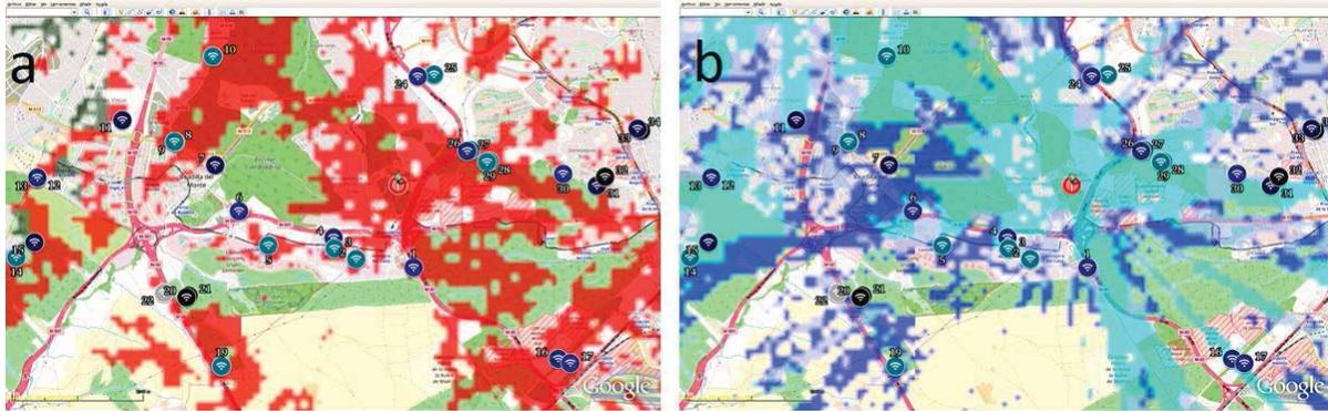
Figure 4. Correlation between simulation and real results: LoS model in a, RSSI for SF=12 model in b. Gateway represented by a red point, light blue points indicates higher PDR while dark blue points represent more packet losses.
