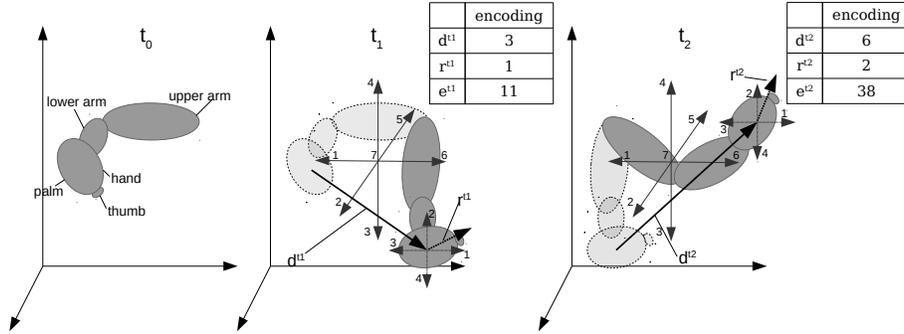
Figure 3. Example of encoding of two movements of a right arm, from  $t_0$  to  $t_1$  and from  $t_1$  to  $t_2$ . At every instant  $t_i$ , the displacement of the hand is encoded with the  $d^i$ , the rotation of the hand is coded with  $r^i$  and the final encoding, computed using the Cantor pairing function, is represented by the symbol  $e^i$ .
