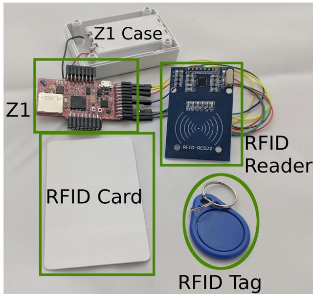
**Figure 1. The hardware setup: The RFID reader is connected to the Z1 sensor node using jumper wires. RFID tags are used to configure the Z1 node.**
