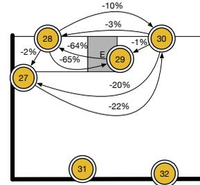
**Figure 12. Links affected by the presence of the elevator at the same floor. The link demonstrating a change in PDR are depicted with the corresponding quality change.**
