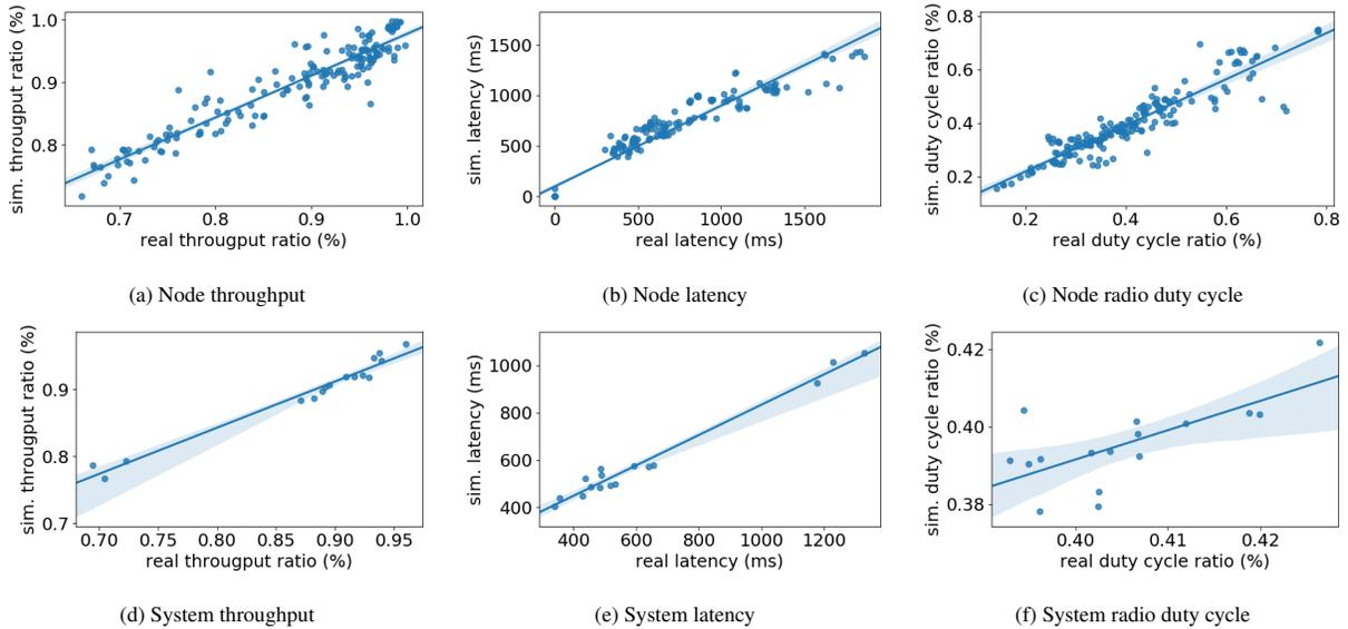
**Figure 6. Linear regression and 95% confidence interval for the relationship between simulated metrics and corresponding real performance for all analysed network configurations.**
