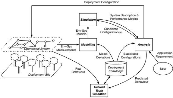
**Figure 2.** *Mορφεύς* framework and its use for deployment and reconfiguration planning.
