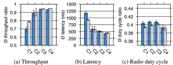
Figure 1. Application metrics for different real-life configurations (blue) and corresponding simulations (gray).
