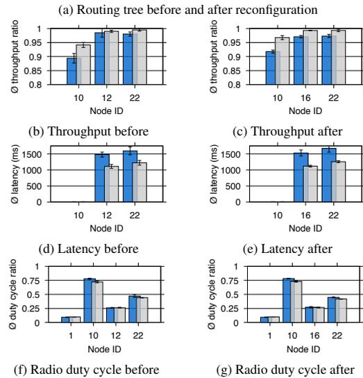
**Figure 8. Behaviour of a network with a weak link before and after the replacement of a node.**
