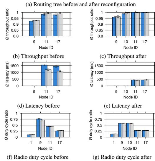
**Figure 10. System behaviour of a network with high latency before and after the addition of a node.**
