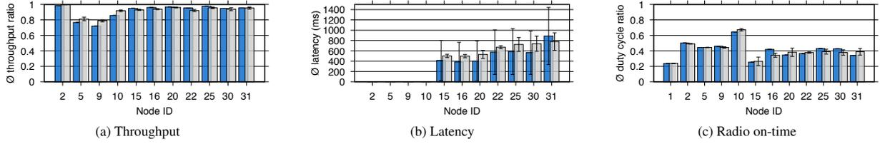
**Figure 7. Node-level application metrics for simulations (grey) based on real-world measurements and same boot order of nodes in comparison to the reference real-world system performance (blue) for configuration C6.**
