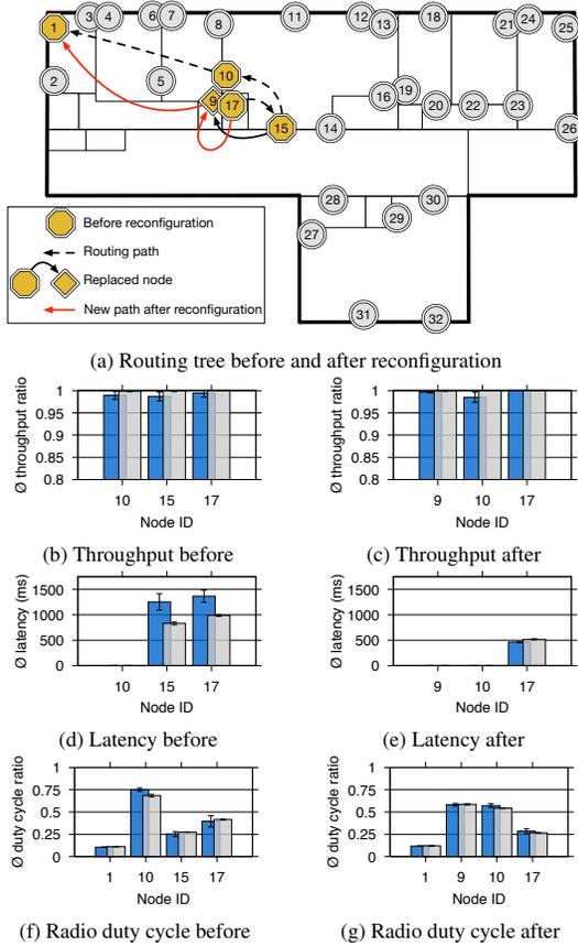
**Figure 11. System behaviour of a network with high latency before and after the replacement of a node.**
