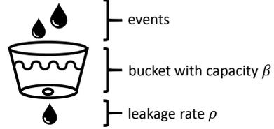
Figure 2. Intuition behind leaky bucket counters
