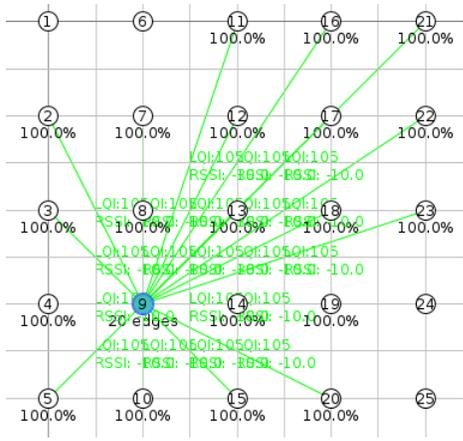
**Figure 7.** Network topology with a hidden wormhole between {3, 4, 5, 9, 10, 15} and {11, 16, 17, 21, 22, 23}
