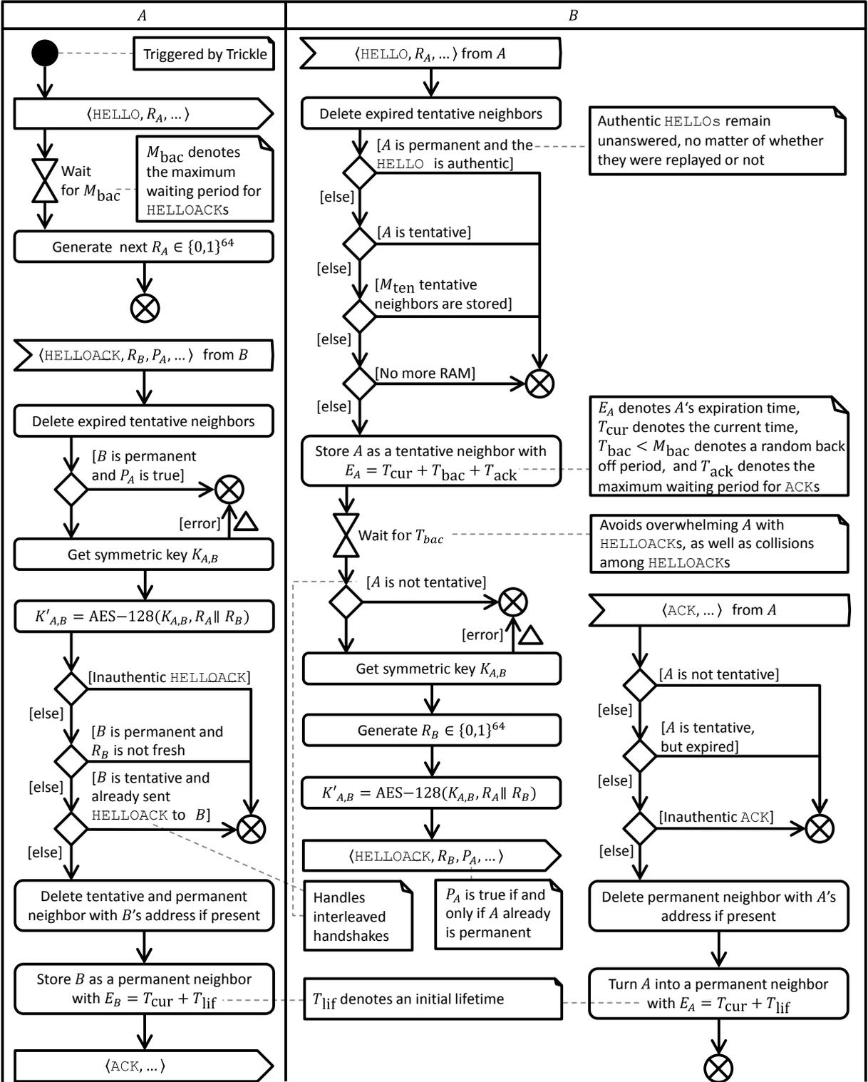
Figure 1. Detailed instructions for processing HELLOs, HELLOACKs, and ACKs
